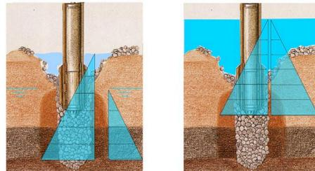
Figure 2. Differential water head for onshore and offshore installation, , adapted from Al-Homoud and Degen (2006)
