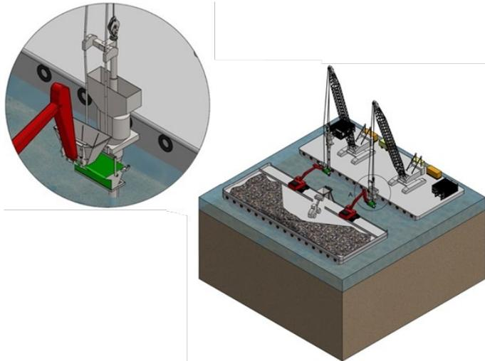
Figure 12. Variant with skip bucket rig and secondary barge
