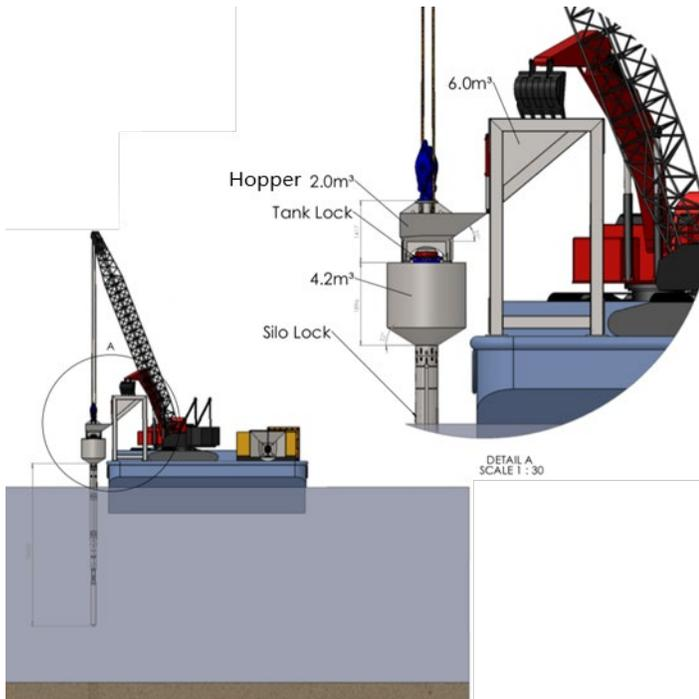
Figure 15. Equipment for single feeding cycle
