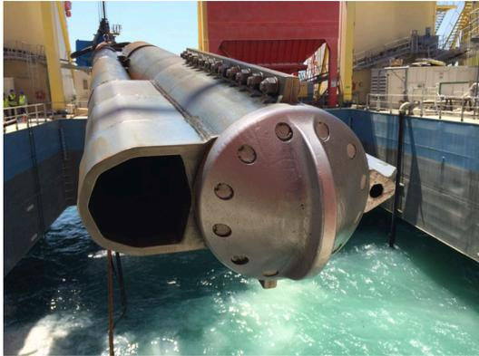
Figure 8. Vibroflot with nose cone, tremie pipe and water jet pipe
