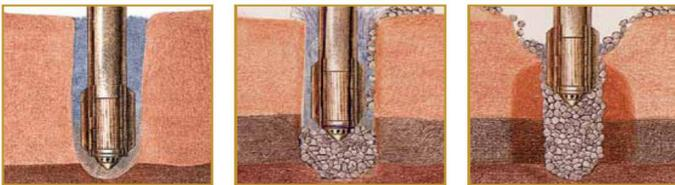
Figure 1. Wet Top Feed installation
