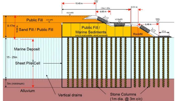
Figure 6. HKBCF typical seawall section (Arup Website, 2019)
