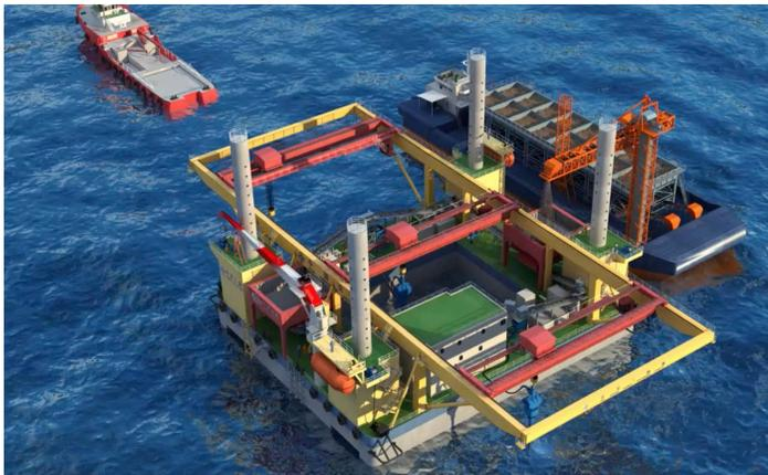
Figure 16. Jack up platform to work in open water
