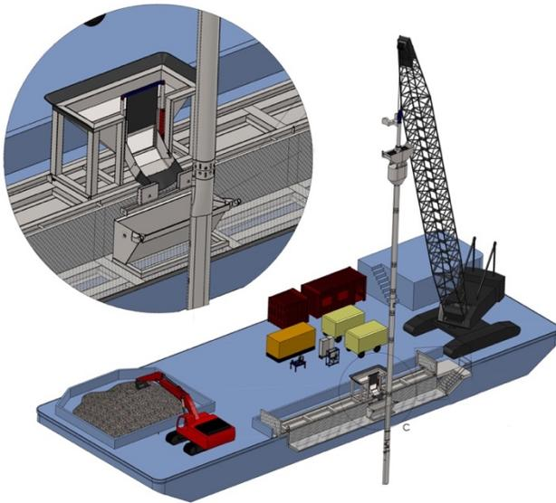
Figure 11. Feeding system with skip bucket
