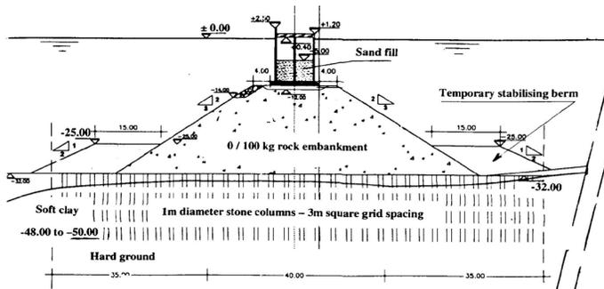
Figure 4. Typical breakwater section in the Harbour of Patras, adapted from Debats and Degen (2001)
