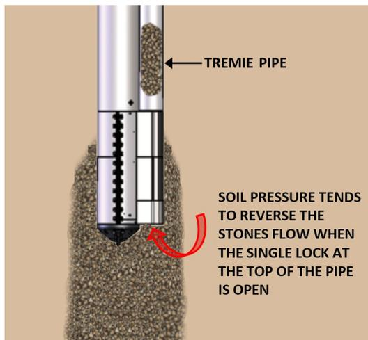
Figure 9. Stones feeding with single lock system
