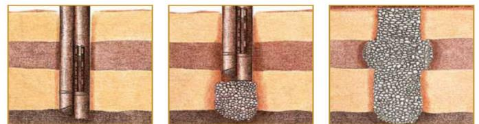
Figure 3. Bottom Feed installation
