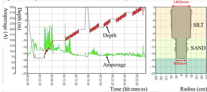
Figure 22. Variable diameter columns in layered soil
